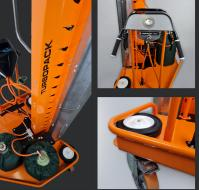
The Turbopack is a mobile heating column, loaded on an easily movable trolley. It gives the operator the possibility to heat-shrink his load anywhere in the shipping area, very useful to avoid the movement of unstable loads.
